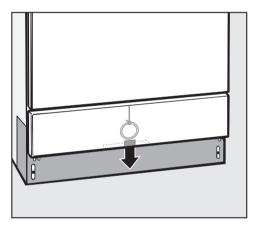
■ Reach behind the service panel and pull the ring of the emergency release downwards.
